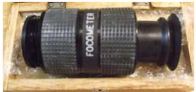
**Figure 2. The Focometer**
