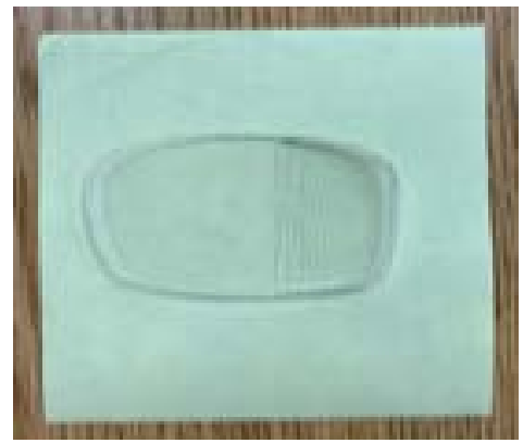
Figure 7. Line up the edge of the Fresnel prism with the vertical line drawn on the lens with removable marker. Cut the Fresnel prism to fit the shape of the lens.
