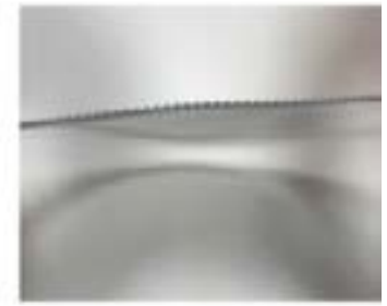
Figure 10 (right). Press-on Fresnel prism highlighting the 1mm multiple prisms that make up a press-on Fresnel prism.
