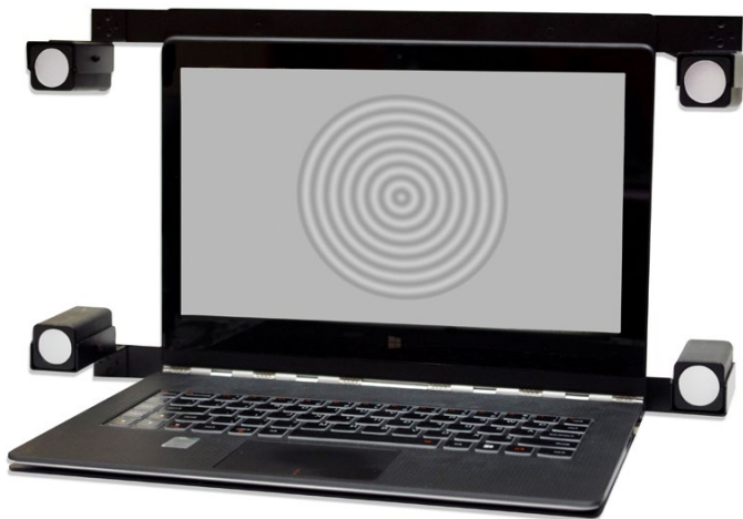
Figure 1. The system used, with one of the sinusoidal bull's-eye CS targets shown. The four outboard lights provide the glare source; luminance was calibrated with a lux meter at the plane of the face of the subjects.
