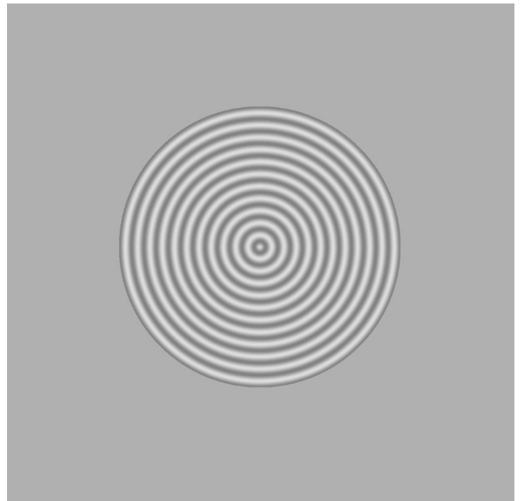
Figure 6. Sinusoidal bull's-eye target on the screen as it appears to the test subject. The target shown here is the 12 cycles per degree target.
