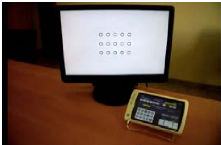
Video 1. Haase method stereo acuity test for vertical disparity, similar to the Landolt ring version seen on the AOC Polar chart
