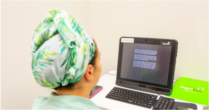
Figure 3. Tobii eye tracking video system assessing reading eye movements
