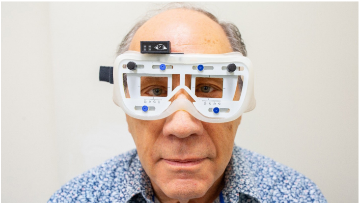
Figure 2. Infrared limbal eye movement system
